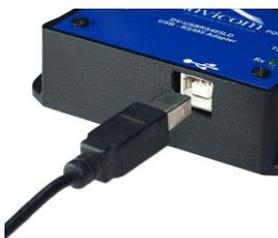
6. Connect the other end of the USB cable to the USB connector located on the rear panel of the Davicom unit.
